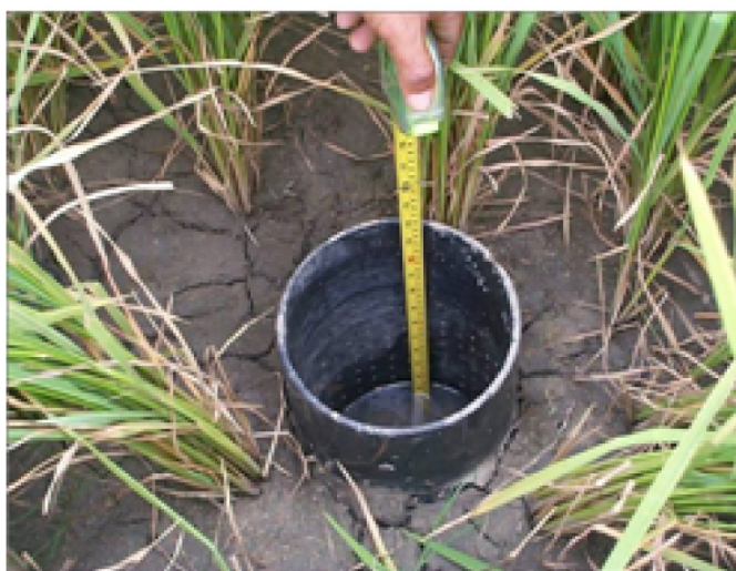
Figure 3.8 Alternate wetting and drying (AWD) technology for methane mitigation. The water table level has been lowered to the stress stage (15cm depth) so that it is time to flood the field again.
